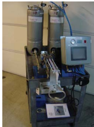
Glenmarc meter/mix/dispense machine with color touch screen PLC potting electronics parts for Raytheon Missile Co..
