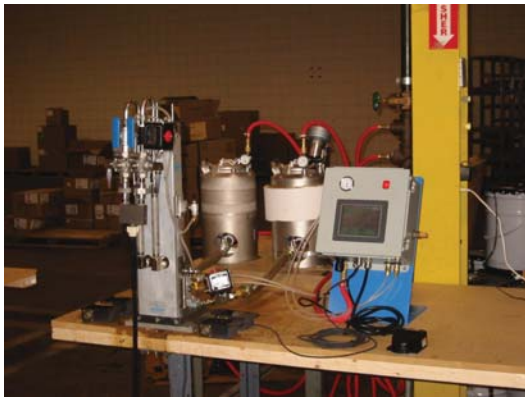
Glenmarc meter/mix/dispense machine with color touch screen PLC potting electronics parts for military Hummers at Swiss Controls.
