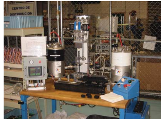
Glenmarc meter/mix/dispense machine with color touch screen PLC potting electronics parts for smoke detectors for System Sensor Honeywell Corp.
