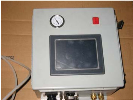
Front view of screen/PLC enclosure
